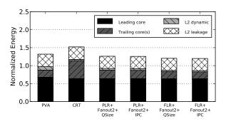
**Figure 5** – Component-wise energy consumption breakdown for the architectures evaluated across all the benchmarks.
