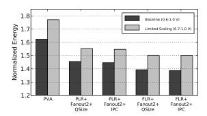
Figure 8 - Impact of limited voltage scaling
