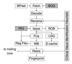
Figure 2 - An RECVF processor core.
