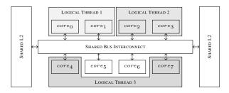
Figure 1 - CMP Block Diagram
