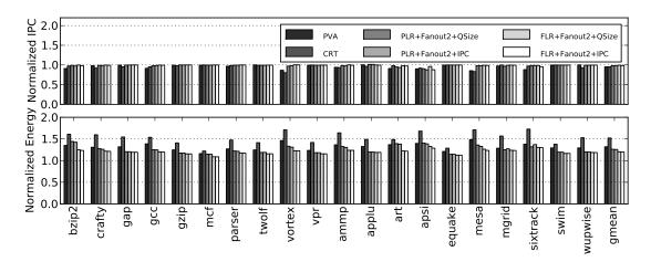
Figure 4 - Normalized IPC (above) and normalized energy (below) of the shared L2 configuration
