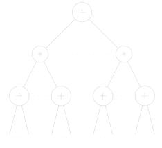
For identity testing, it is sufficient to consider a "sum of product of linear functions" (ΣΠΣ circuit).
