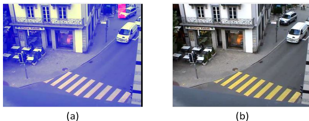
Figure 7: (a) shows car on sidewalk as anomaly in block based method while when ViBe was used it is not the case as seen in (b)
