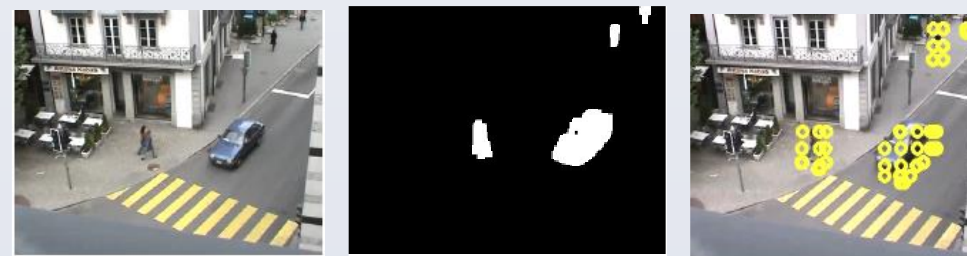
(a) Sample Frame (b) Foreground Marked (c) HOG-HOF Marked Image Source: [4]
