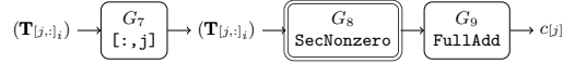
Fig. 7: An abstract diagram of Step 2 in SecRowEch (Algorithm 6). The t -NI gadgets are depicted with a single border and the t -SNI gadgets with a double border.
