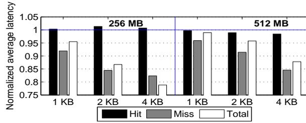
**Figure 27.** Normalized read hit, read miss, and overall average read latency of the Micro-sector cache at 256 MB and 512 MB capacity.
