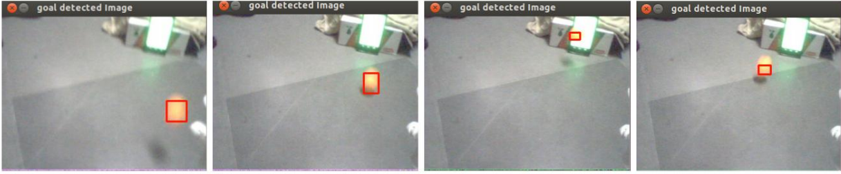
Fig. 7: Detecting where ball bounced. It is visible here that the ball must have bounced first time between frame 2 and 3.
