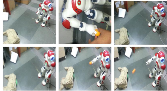
Fig. 8: Sequence of images showing the working of the ball throwing humanoid robot
