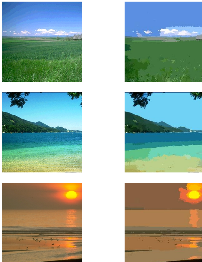
Figure 2: Colored image and its mean shift based segmentation
